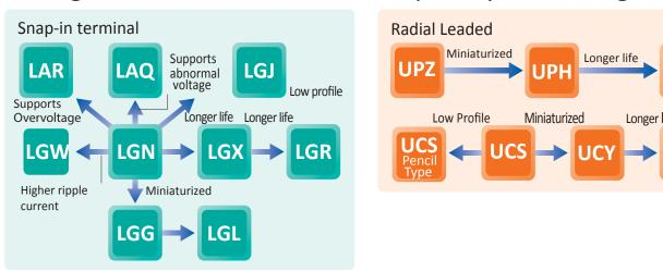
2 Diagram of series recommended for secondary side filtering
